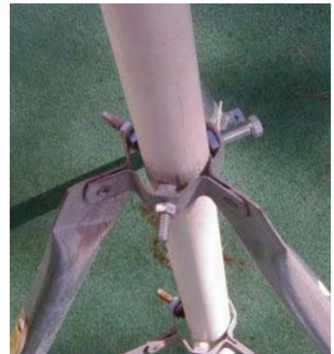
The tripod is great for finding an opening in the trees.... make sure that you have some extra cable along so that you can reach over to that clearing that you've found. I keep a 75 foot piece of RG6 cable for those times when the dish needs to be "way over there".
