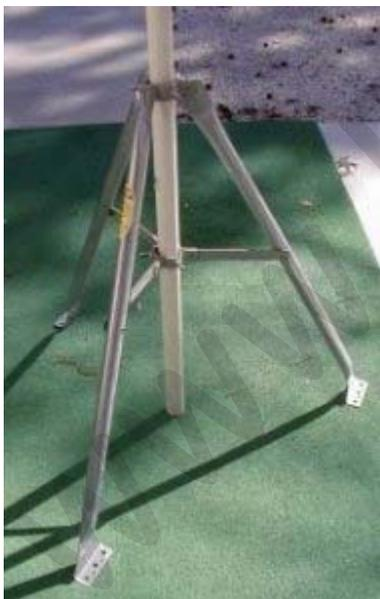
Here are some close ups of my home-made tripod. Using the hardware and goodies that came with the antenna mount, I was able to devise a simple clamp to keep the pipe in place. It folds up nicely for storage when not in use.
