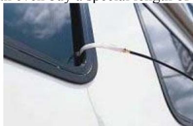
A neater way to do it is to install a cable connector permanently in the side of your rig, or in a compartment. There are many easy to install, weather proof connector jacks available... here are a few common ones.
