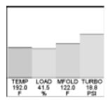
The MultiBar is customized very much like the Scan Gauge. Right-Click on the gauge to bring up the MultiBar Properties box. You may select as many parameters as you wish from the list at the top of the dialog box. You may choose whether to display the Gauge Name (the name is always abbreviated), the Value, and the Unit.
