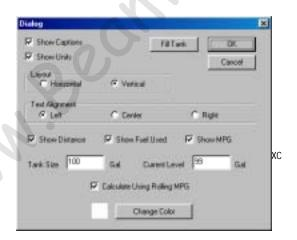
If your tank is not completely filled, or you wish to compensate for fuel burned by other devices, you can adjust the Current Level as needed.
