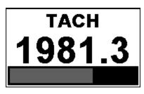
A Simple Gauge consists of a panel with up to four elements. At the top of the panel is the name of the item being displayed and a warning "lamp" that changes from green to yellow to red according to the status of the reading. The middle of the panel shows the value, and the bottom of the panel is a bar graph that provides a "analog" reading.
