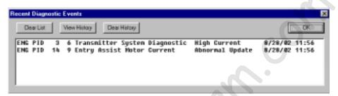
Each line of text shows a fault event. The first column shows the source (Engine, Transmission, or ABS Brakes). The next three columns are used by mechanics to find information in their service manuals. The main part is the plain-language description, which indicates the component that is malfunctioning and the type of malfunction. Finally, the date and time of the first occurence is given.
