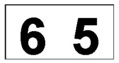
This is one of the simplest gauges. You may choose to show either or both the Gear Selected and the Gear Attained. The Gear Selected will show "6" when you put it into "Drive", but it will automatically change when the engine brake is activated or if you press the Down or Up arrows on the shift console. The Gear Attained shows the gear the transmission is actually in.
