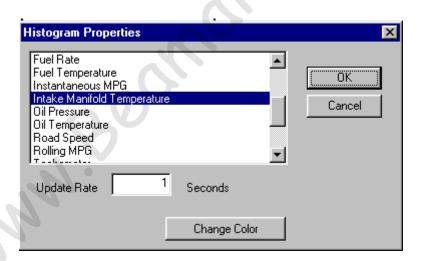
The settings are few and simple. Right-Click on the Histogram to bring up the Histogram Properties box. Select as many parameters as you wish to graph - there is no limit. The Update Rate determines how much time passes between each "tick" - the graph shows 60 ticks. As with all gauges you can control the background color. The color of each graph item, though, is automatically assigned.
