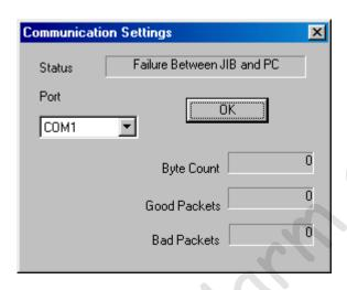
The only user setting here is the Port, which allows you to choose the serial port which the J1708 Interface Board ("JIB") is attached to. If no data is coming from the vehicle, this is the setting you must adjust.
